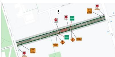
The street closure is required to enable the safe operation of a mobile crane on the roadway in order to hoist materials onto the Ferguson Tower roof.
